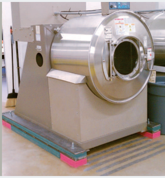
Elastic decoupling of an industrial washing machine
